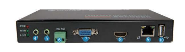
4, Audio output5, Audio line in6, RS-485 Interface7, VGA IN8, HDMI IN9, 100M Ethernet interface10, USB interfaceVersion 1.1 © Changsha KILOVIEW Electronics CO.,LTD. All rights reserved
