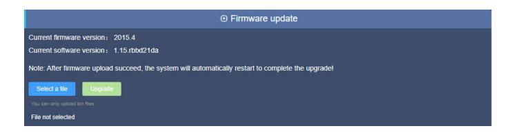
After upgrading, click *at the upper right corner of the WEB page to confirm whether the current software version and the latest upgrade package are the same, to make ensure the device upgrading is successful.*
