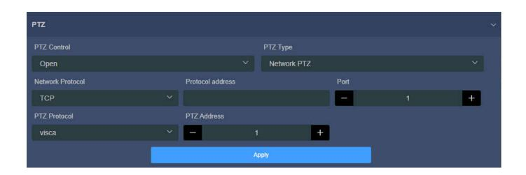
A USB to RS232/RS422/RS485 adaptor is required through TYPE-C to USB. Inserting the USB to RS232/RS422/RS485 adaptor, the device supports PTZ control over serial port.
