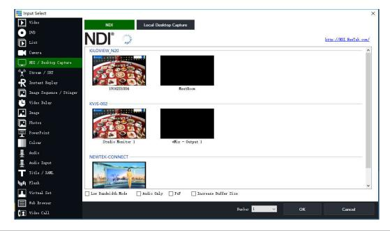
Note: NDI discovery is implemented through multicast. Therefore, the NDI converter and other NDI devices should be in the same subnet. The device is configured with the IP address of the same subnet and can communicate with each other (It can be obtained automatically). Otherwise, NDI stream may not be automatically discovered NDI stream.
