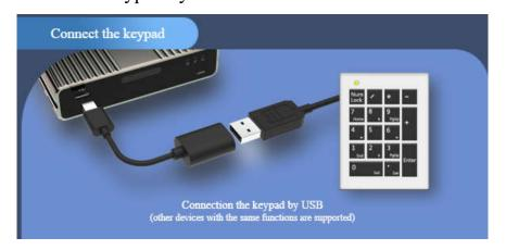
Press [NumLock] on the keypad, if the light is on, you can operate the decoding switch. Press 1~9 to select the corresponding 1~9 preset decoding source, and press 0 to select blank output.
