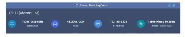
Click on the right, you can configure the output parameters. The resolution of decoding output will be the same as that of the source. Frame rate and audio sample rate can be set accordingly.
