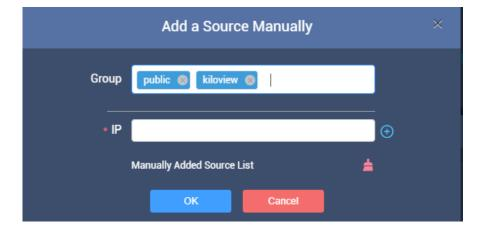
When you need to search for NDI sources across network segments, if the group name is a non-public group, you need to fill in the specified group name firstly, and then fill in the specified IP address in the "IP" box, click the button , this IP address will be added to
