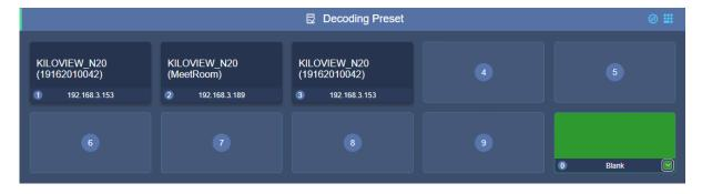
There is a blank output box in decoding preset, if switching to a source without video output, the device will output the set color. It can also be used for testing the output to the monitor by choosing a different color.
