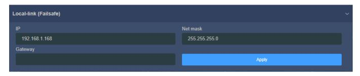
"Failsafe" is to bind the device to an independent IP address. This IP address does not affect the use of other network cards. In special cases, it can be used to manage the encoder. This address can be changed manually (Usually no need to change), the default address is 192.168.1.168.
